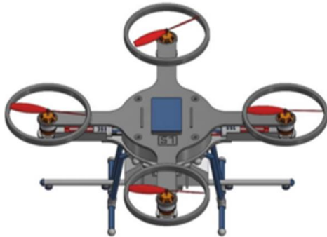
Figure 4: Top view of a designed quadcopter model on CAD Inventor
