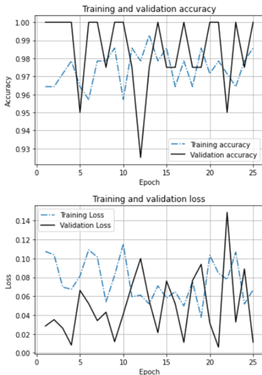
Figure 14: Graph representation of Training and Validation accuracy and loss of ResNet50 model
