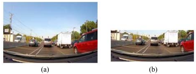
Fig. 3 (a) RGB image and (b) the cropped rectangular image based on points of a line detect by Hough transform
