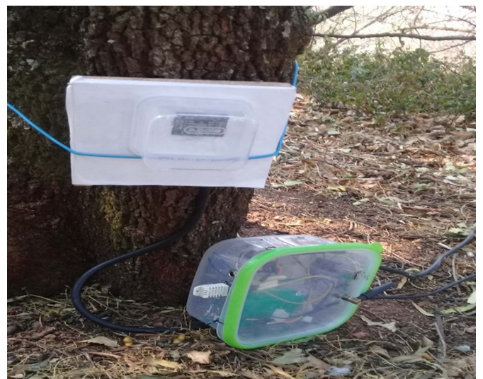
Figure 6: Circuitry box and the TCS3200 color sensor
